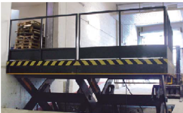
Double scissor lift with hydraulic lip and railings and folding doors
