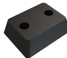
DB330-100RB 330 Rubber Dock Bumper Material: Natural SBR Rubber Unit: Piece (1) Dimensions: 330(H)x250(W)x100(D)
